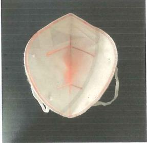
Artificial blood has not passed into the inner surface of the mask.
